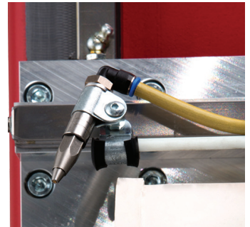
Minimal lubrication system extends tool life without creating a mess
